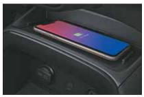
For charging a compatible smartphone wirelessly on the pad
