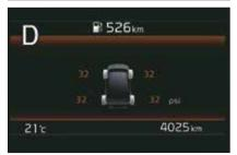
Continuously monitors air pressure in each tyre and alerts you in case of a drop below recommended levels while driving
