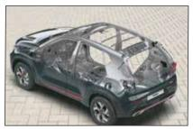
Offers enhanced safety as more than 2/3<sup>rd</sup> of structure is made from high strength steel
